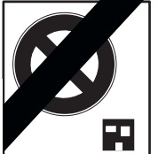
E15 End of zone with limited parking time.
