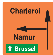
F39 Advance direction sign indicating there is a diversion ahead.
