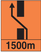
F83 Advance direction sign indicating a crossing of the central reservation ahead.
