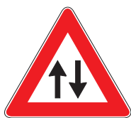
A39 Two-way traffic after a road section with one-way traffic.
