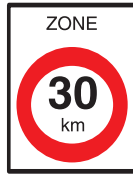
F4a Beginning of a zone with a speed limit of 30 kph.
