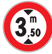
C29 No entry for vehicles of which the height, including load, is in excess of the height shown.
