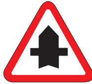
B15 Priority. The horizontal line may be altered to give a better idea of the layout of the roads.
