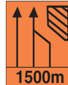
F79 Advance direction sign indicating a reduction in the number of traffic lanes.
